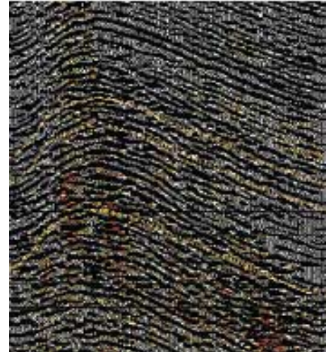
Figure 6b: Estimated crack density overlaid by the estimated shear-wave stack. The shear-wave stack is estimated using the AVO method of Gidlow et al (1992).
